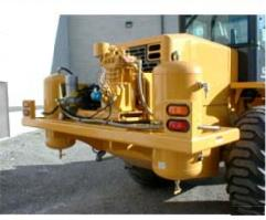
For non-hi-rail applications the front or rear mount Railcar Coupler makes a good choice. The coupler can be free float left or right in the manual alignment bumper. The coupler can be mounted on the front through a quick coupler or permanently mounted on the rear frame of the machine.
