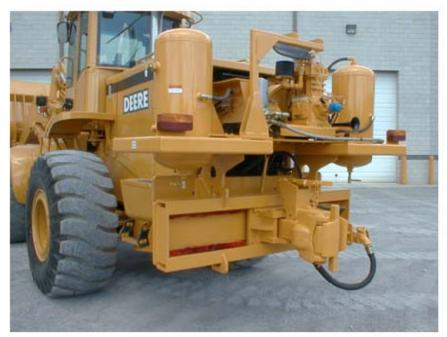
From the operators cab, power the coupler left or right, release the coupler pin and control the railcar brakes.
